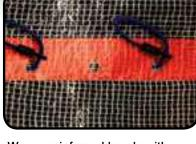
Woven reinforced bands with perforated eyelets
